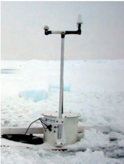
Telemetry buoys or tracking buoys can be used to acquire and transmit data from different scientific instruments or just for tracking the instruments position or any other target like an iceberg.
