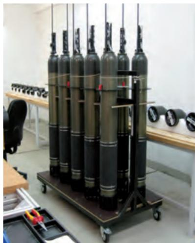
The *NEMO*-Float is based on the SOLO design and has been further improved to allow also the deployment under ice, the positioning through GPS and RAFOS as well as the integration of new sensors.
